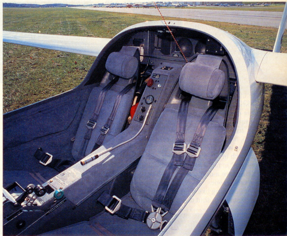
The Stemme's pop-open nose cone lets a spring-loaded folding propeller extend for powered flight. Hinged wing panels swing back for easy storage. The cockpit is snug, but comfortable, and sports a nonstandard panel, control stick-mounted brake levers, and two variometers.
