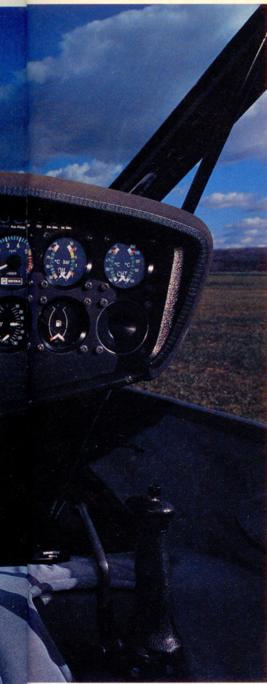
The Stemme's pop-open nose cone lets a spring-loaded folding propeller extend for powered flight. Hinged wing panels swing back for easy storage. The cockpit is snug, but comfortable, and sports a nonstandard panel, control stick-mounted brake levers, and two variometers.
